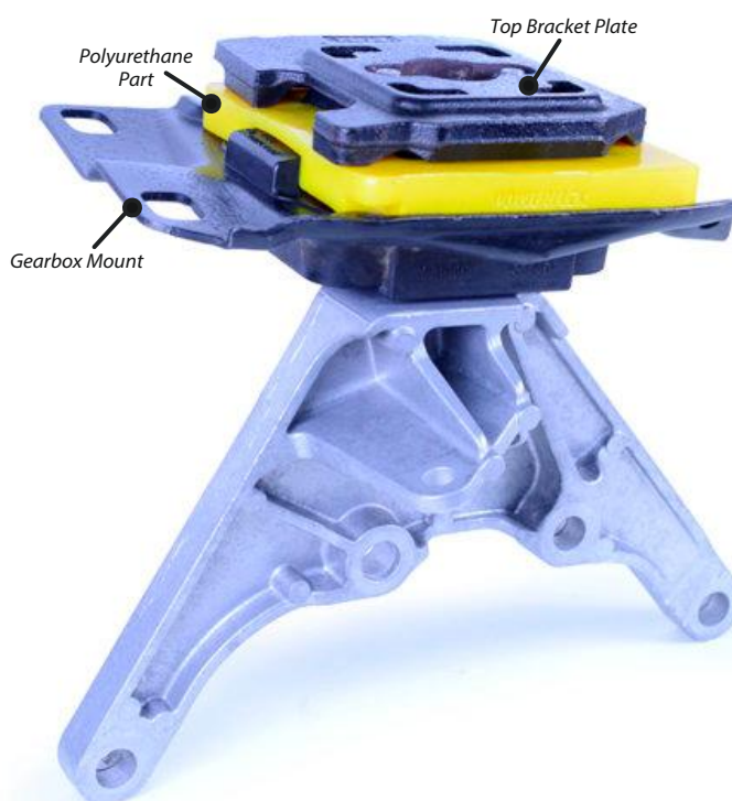
Figure 1 - fitted image of the polyurethane part inside the gearbox mount
